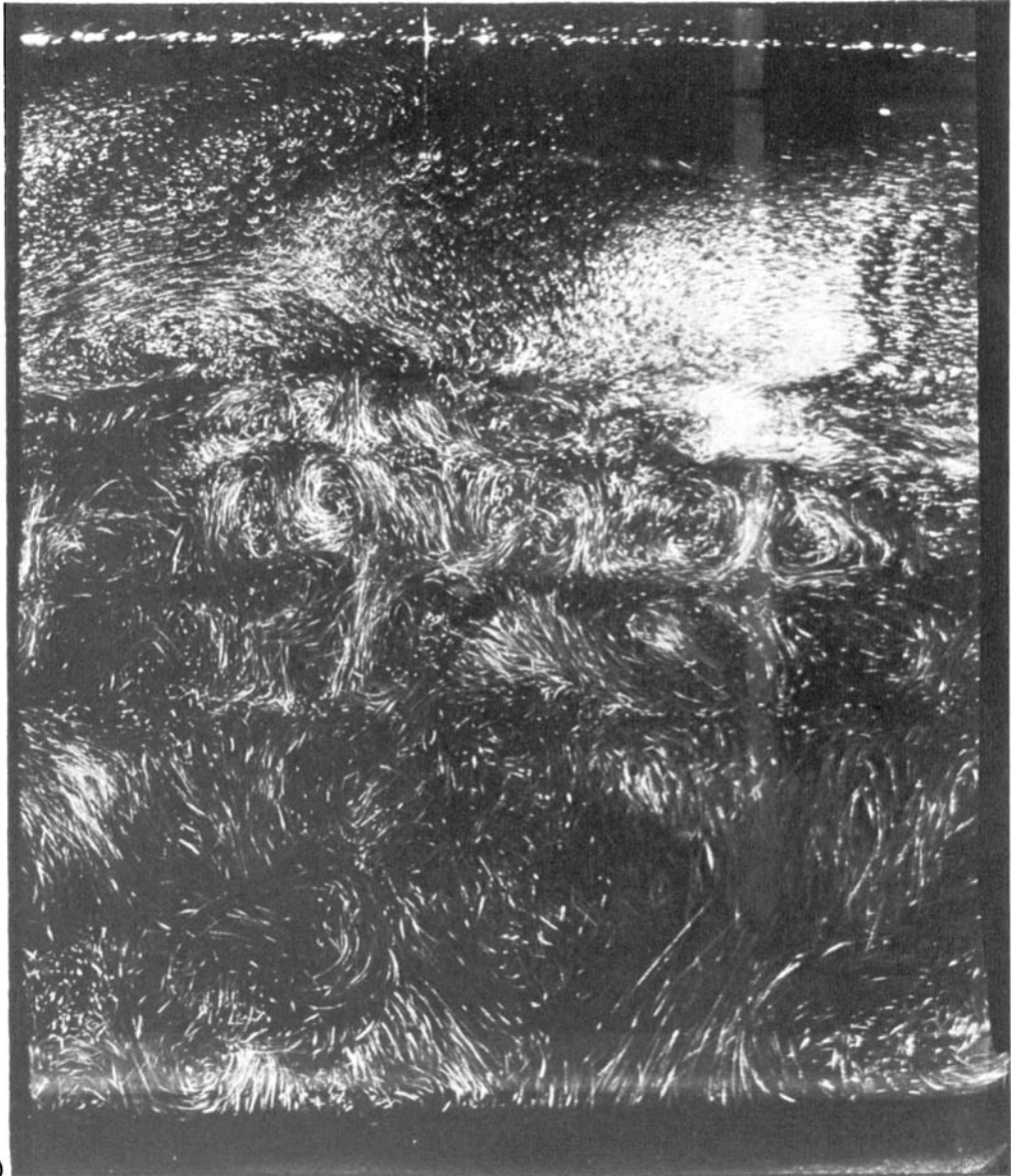
FIGURE 5. Time exposures of aluminium particles suspended in the flow. (a) An intermediate stage in the experiment showing about 3 layers. Length of exposure 3 s. (b) A later stage in the same experiment with 4 layers. Length of exposure 10 s. Both photographs also show evidence of internal wave motion above the convecting region. The flow is illuminated by a vertical slit of light 1 cm thick and is viewed normal to this beam. The full depth of the tank (25 cm) is visible, except for a region 1.5 cm deep directly above the base.
