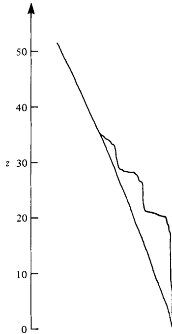
FIGURE 8. Two conductivity profiles taken before and 36 min after the start of an experiment. The profiles are plotted without adjustment and we note that above the convecting region the salinity gradient is unaltered from its original value.
